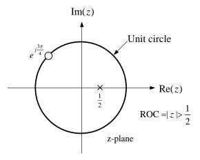
Determine the z-transform of each of the following signals in terms of X(z). Sketch the pole-zero plot and indicate the ROC for each case.
