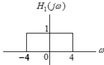
From the above figure, we can see that the  $h_1(t)$  is an ideal low-pass filter with passband  $|\omega| \leq 4$ . Therefore,  $h(t)$  can be seen as the impulse response of an ideal low-pass filter shifted by one to the right. Using the shift property, we have
