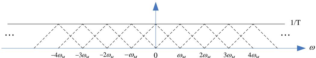
$x(t)$  can't be reconstructed from  $x_p(t)$  due to the aliasing in  $X_p(\omega)$ .
