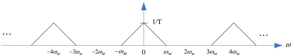
$x(t)$  can be reconstructed from  $x_p(t)$  since there is no aliasing in  $X_p(\omega)$ .
