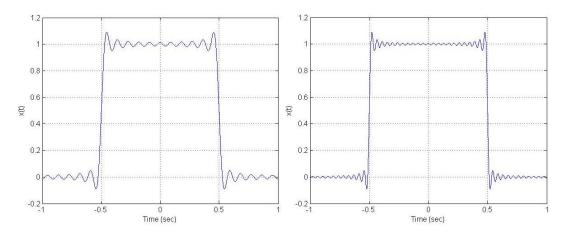
Note that as N increases, the *ripples* in the approximating waveform  $x_N(t)$  get narrower and narrower, but the *overshoot* of the waveform beyond the desired unity amplitude remains constant at about  $\pm 0.18\%$ , or about 9% of the height of the discontinuity.
