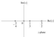
In the case, identify the valid ROC for X(z), and specify whether the time signal corresponding to the ROC, is right sided, left sided or two-sided.
