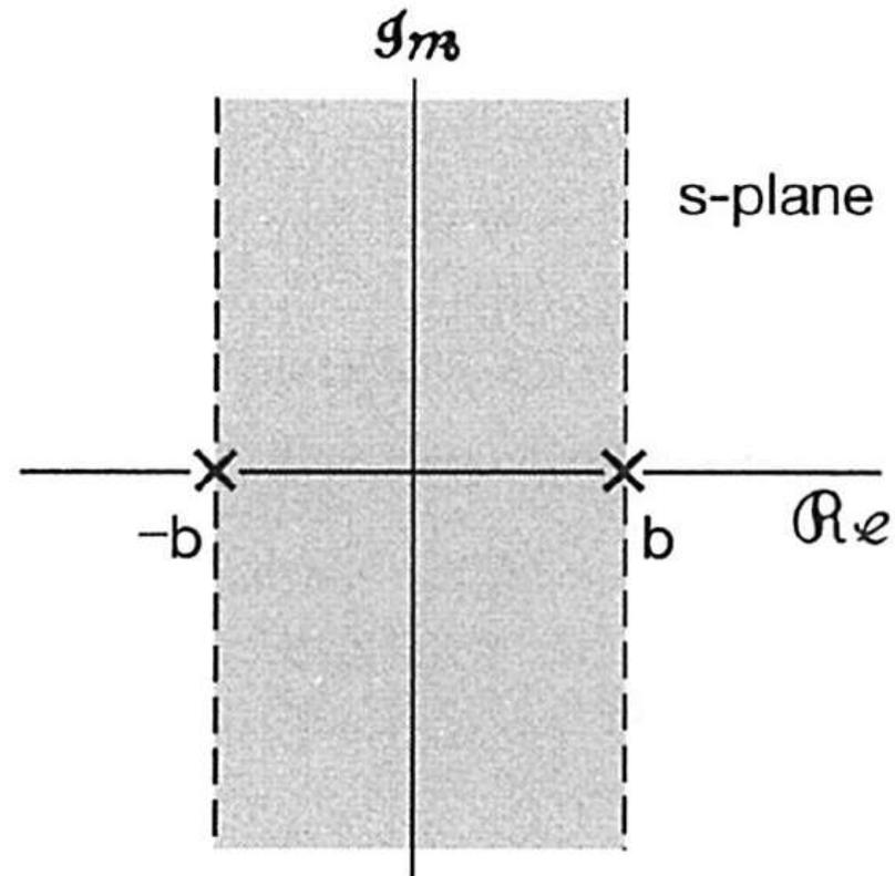
**Figure 9.12** Pole-zero plot and ROC for Example 9.7.
