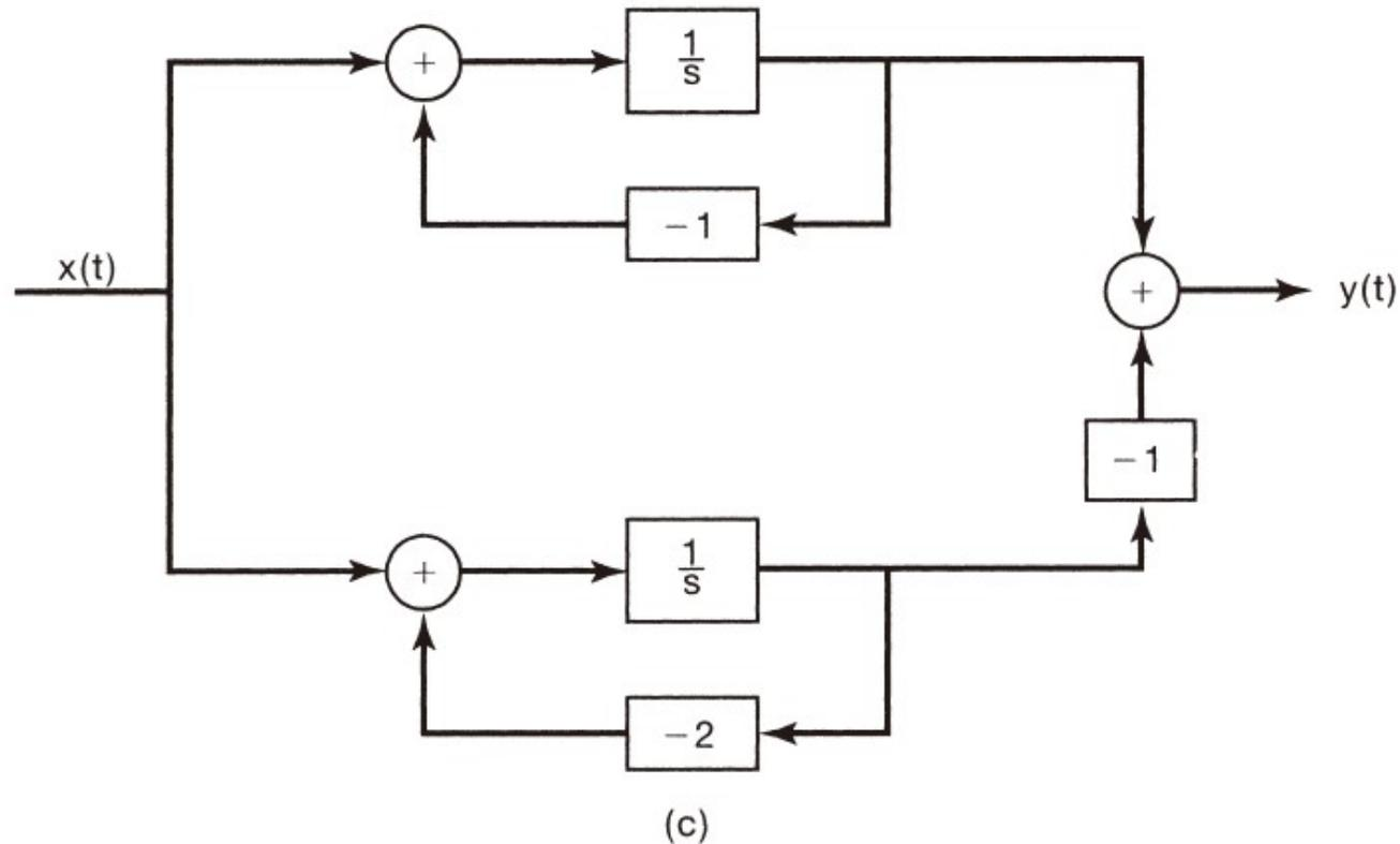
Alternatively, by performing a partial-fraction expansion of  $H(s)$ , we obtain
