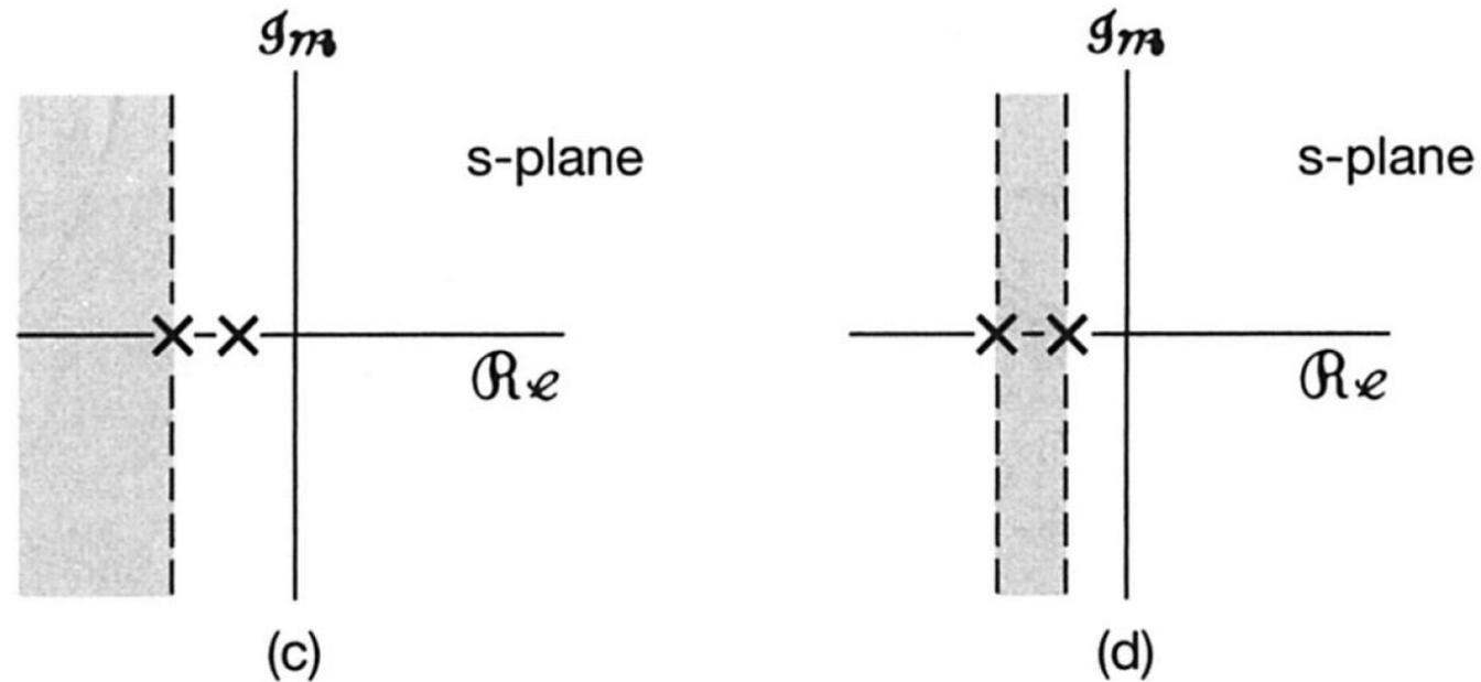
**Figure 9.13** (a) Pole-zero pattern for Example 9.8; (b) ROC corresponding to a right-sided sequence; (c) ROC corresponding to a left-sided sequence; (d) ROC corresponding to a two-sided sequence.
