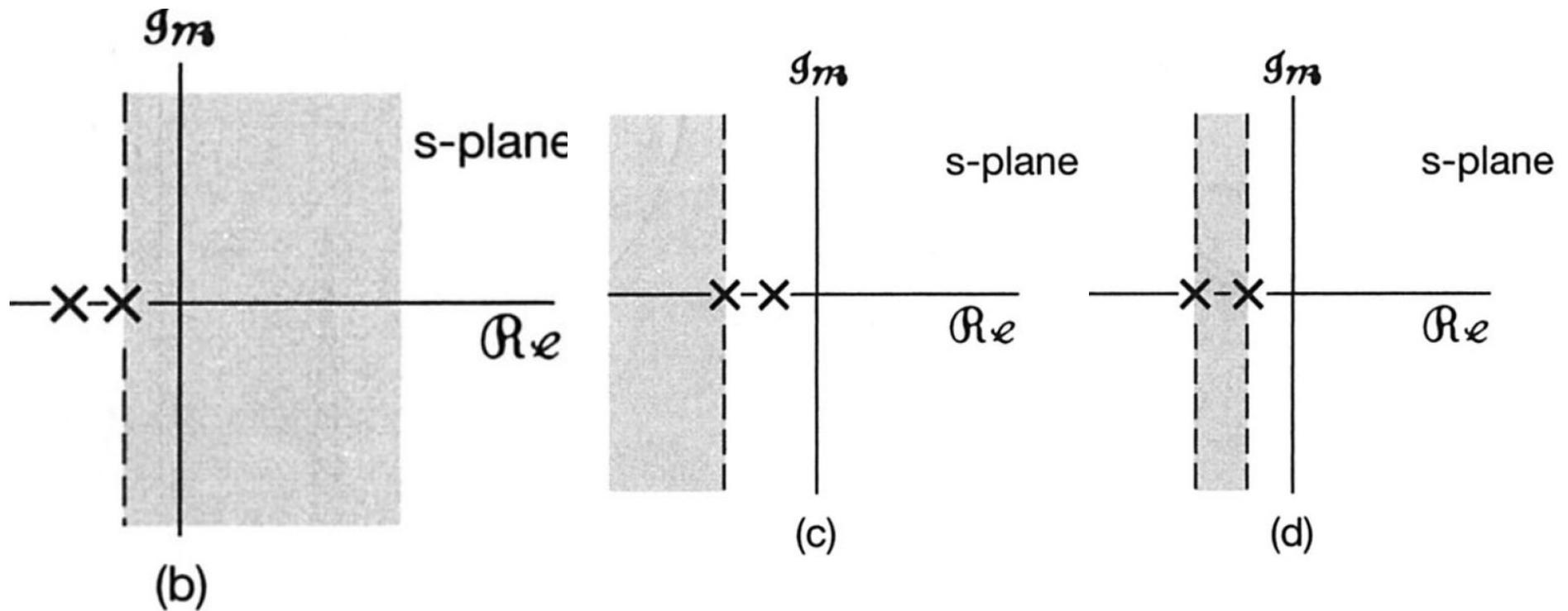
For Figure 9.13(b), since the ROC includes the  $j\omega$ -axis, the Fourier transform of this signal converges. Figure 9.13(c) corresponds to a left-sided signal and Figure 9.13(d) to a two-sided signal. Neither of these two signals have Fourier transforms, since their ROCs do not include the  $j\omega$ -axis.
