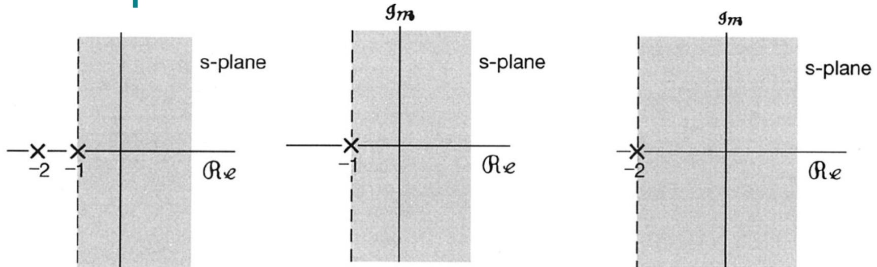
(a) Since the ROC for  $X(s)$  is  $\Re\{s\} > -1$ , the ROC for the individual terms in the partial-fraction expansion of eq. (9.62) includes  $\Re\{s\} > -1$ . The ROC for each term can then be extended to the left or right (or both) to be bounded by a pole or infinity. This is illustrated in Figure 9.14. Figure 9.14(a) shows the pole-zero plot and ROC for  $X(s)$ , as specified in eq. (9.58).
