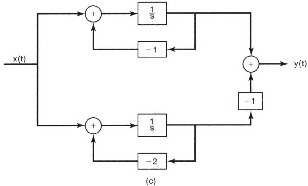
**Figure 9.34** Block diagram representations for the system in Example 9.30: (a) direct form; (b) cascade form; (c) parallel form.
