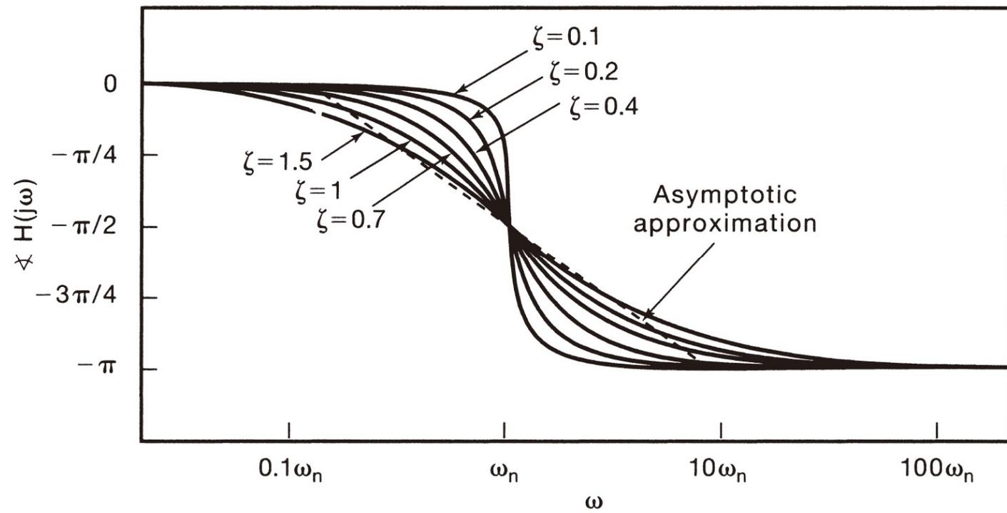
$$H(s) = \frac{\omega_n^2}{(s - c_1)(s - c_2)} \quad \begin{aligned} c_1 &= -\zeta\omega_n + \omega_n\sqrt{\zeta^2 - 1}, \\ c_2 &= -\zeta\omega_n - \omega_n\sqrt{\zeta^2 - 1}, \end{aligned}$$
