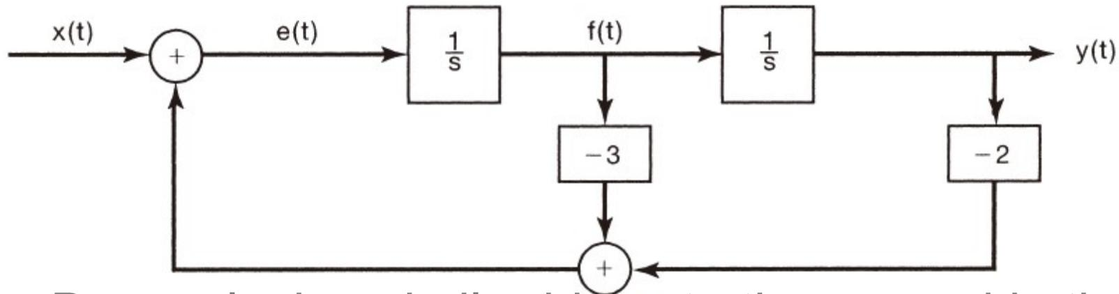
By employing similar ideas to those used in the preceding examples, we obtain the block diagram representation for this system shown in Figure 9.34(a). Specifically, since the input to an integrator is the derivative of the output of the integrator, the signals in the block diagram
