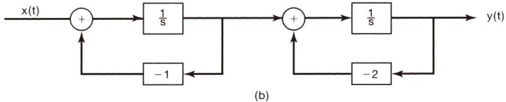
The block diagram in this figure is sometimes referred to as a **direct-form** representation, since the coefficients appearing in the diagram can be directly identified with the coefficients appearing in the system function or, equivalently, the differential equation. Other block diagram representations of practical importance also can be obtained after a modest amount of system function algebra.
