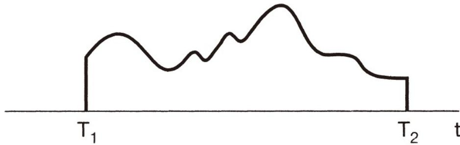
**Figure 9.4** Finite-duration signal.
