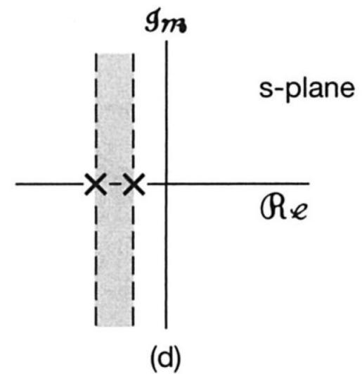
From Examples 9.1 and 9.2, we know that there are two possible inverse transforms for a transform of the form  $1/(s + a)$ , **depending on whether the ROC is to the left or the right of the pole**. Consequently, we need to determine which ROC to associate with each of the individual first-order terms in eq. (9.62). This is done by reference to the properties of the ROC developed in Section 9.2.
