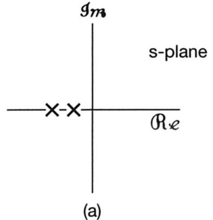
with the associated pole-zero pattern in Figure 9.13(a). As indicated in Figures 9.13(b)-(d), there are three possible ROCs that can be associated with this algebraic expression, corresponding to three distinct signals. The signal associated with the pole-zero pattern in Figure 9.13(b) is right sided.
