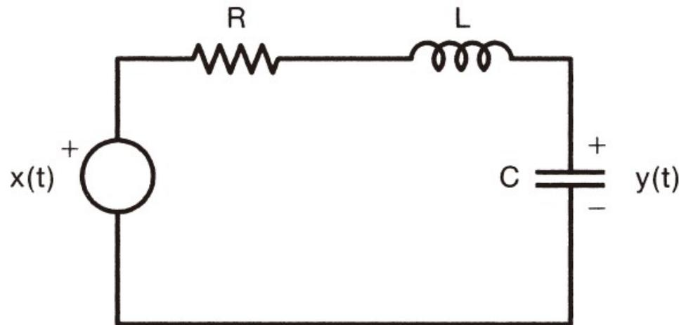
**Figure 9.27** A series  $RLC$  circuit.
