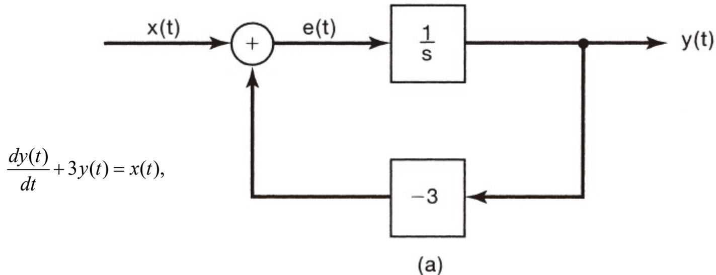
together with the condition of **initial rest**. In Section 2.4.3 we constructed a block diagram representation, shown in Figure 2.32, for a first-order system such as this. An equivalent block diagram (corresponding to Figure 2.32 with  $a = 3$  and  $b = 1$ ) is shown in Figure 9.32(a). Here,  $1/s$  is the system function of a system with impulse response  $u(t)$ , i.e., it is the system function of an **integrator**.
