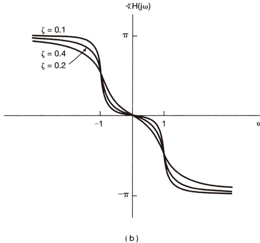
**Figure 9.20** (a) Magnitude and (b) phase of the frequency response for a second-order system with  $0 < \zeta < 1$ .
