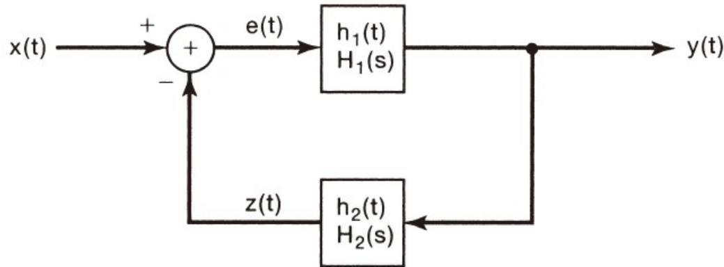
While analysis of the system in the time domain is not particularly simple, determining the overall system function from input  $x(t)$  to output  $y(t)$  is a straightforward algebraic manipulation. Specifically, from Figure 9.31,
