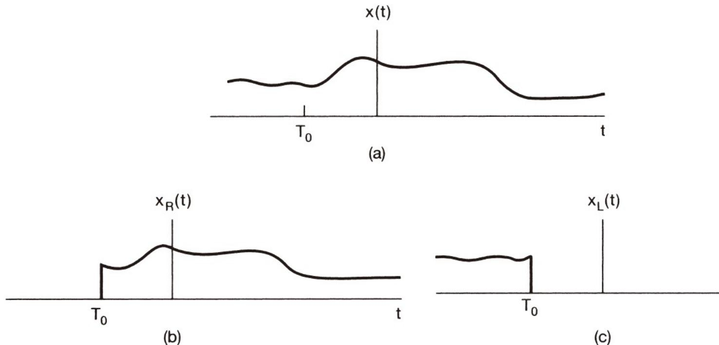
**Figure 9.9** Two-sided signal divided into the sum of a right-sided and left-sided signal: (a) two-sided signal  $x(t)$ ; (b) the right-sided signal equal to  $x(t)$  for  $t > T_0$  and equal to 0 for  $t < T_0$ ; (c) the left-sided signal equal to  $x(t)$  for  $t < T_0$  and equal to 0 for  $t > T_0$ .
