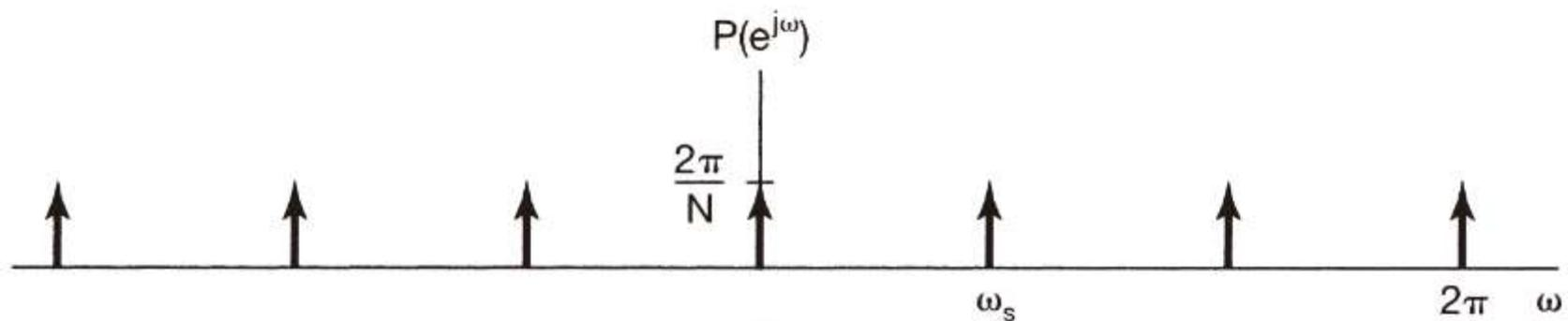
$$X_p(e^{j\omega}) = \frac{1}{N} \sum_{k=0}^{N-1} X(e^{j(\omega - k\omega_s)}). \quad \omega_s = \frac{2\pi}{N}$$
