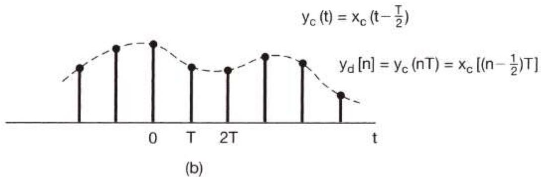
**Figure 7.30** (a) Sequence of samples of a continuous-time signal  $x_c(t)$ ; (b) sequence in (a) with a half-sample delay.
