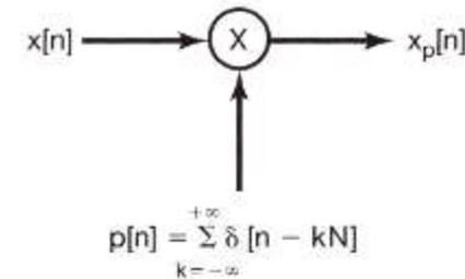
$$(7.39) \quad \begin{aligned} x_p[n] &= x[n]p[n] \\ &= \sum_{k=-\infty}^{+\infty} x[kN]\delta[n - kN], \end{aligned}$$
