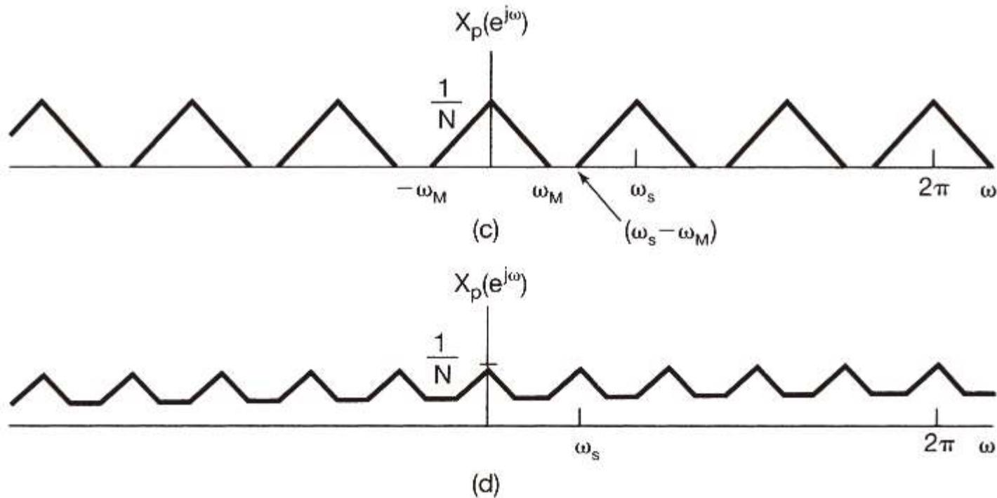
**Figure 7.32** Effect in the frequency domain of impulse-train sampling of a discrete-time signal: (a) spectrum of original signal; (b) spectrum of sampling sequence; (c) spectrum of sampled signal with  $\omega_s > 2\omega_M$ ; (d) spectrum of sampled signal with  $\omega_s < 2\omega_M$ . Note that aliasing occurs.
