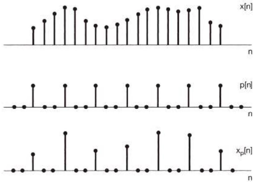
**Figure 7.31** Discrete-time sampling.
