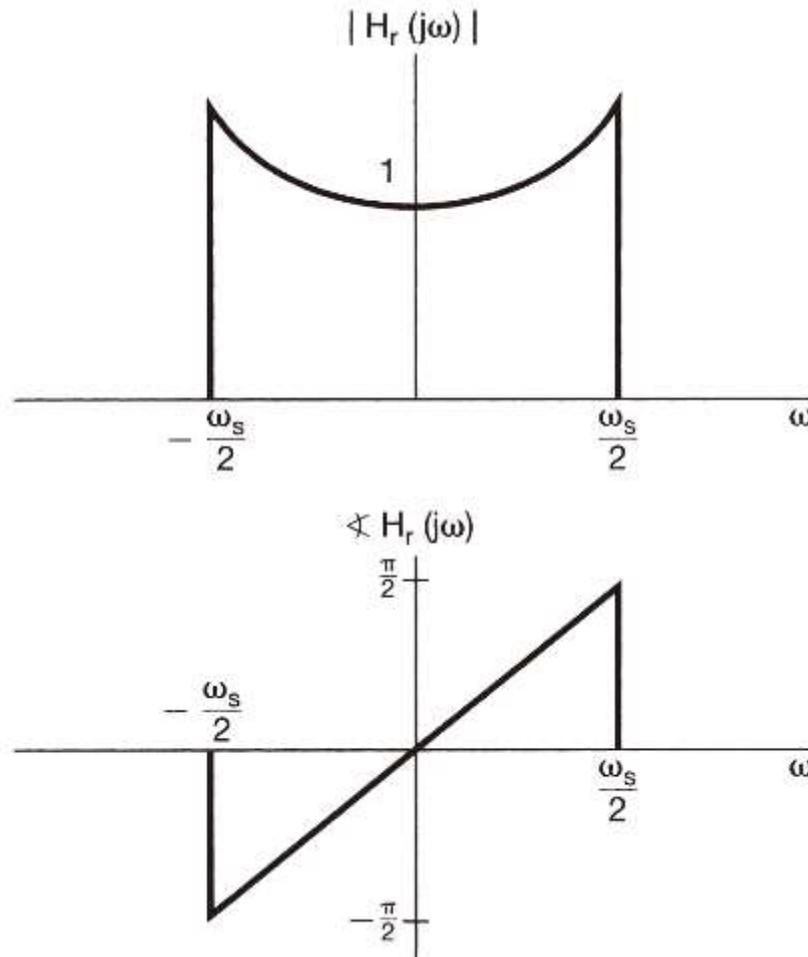
$$H_r(j\omega) = \frac{e^{j\omega T/2} H(j\omega)}{2 \sin(\omega T / 2)} \omega$$
