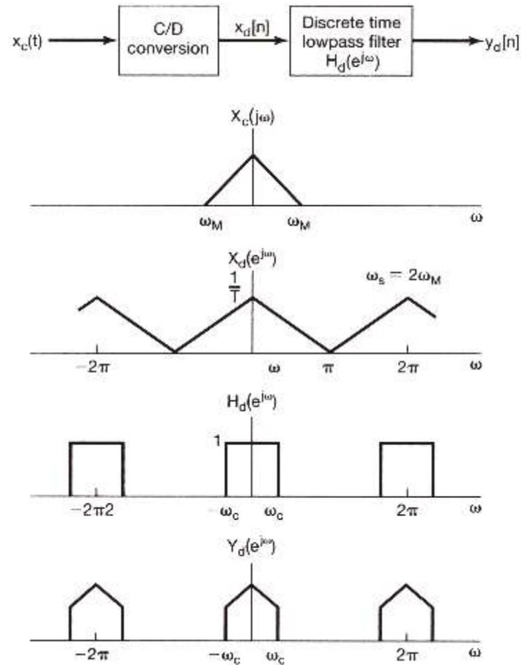
**Figure 7.36** Continuous-time signal that was originally sampled at the Nyquist rate. After discrete-time filtering, the resulting sequence can be further downsampled. Here  $X_c(j\omega)$  is the continuous-time Fourier transform of  $x_c(t)$ ,  $X_d(e^{j\omega})$  and  $Y_d(e^{j\omega})$  are the discrete-time Fourier transforms of  $x_d[n]$  and  $y_d[n]$  respectively, and  $H_d(e^{j\omega})$  is the frequency response of the discrete-time lowpass filter depicted in the block diagram.
