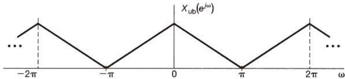
when  $x_u[n]$  is then downsampled by a factor of 9, the spectrum of the resulting sequence  $x_{ub}[n]$  is as shown in Figure 7.38(d). This combined result effectively corresponds to downsampling  $x[n]$  by a noninteger amount,  $9/2$ . Assuming that  $x[n]$  represents unaliased samples of a continuous-time signal  $x_c(t)$ , our interpolated and decimated sequence represents the maximum possible (aliasing-free) downsampling of  $x_c(t)$ .
