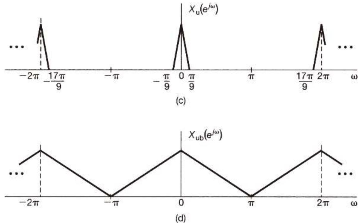
**Figure 7.38** Spectra associated with Example 7.5. (a) Spectrum of  $x[n]$ ; (b) spectrum after downsampling by 4; (c) spectrum after upsampling  $x[n]$  by a factor of 2; (d) spectrum after upsampling  $x[n]$  by 2 and then downsampling by 9.
