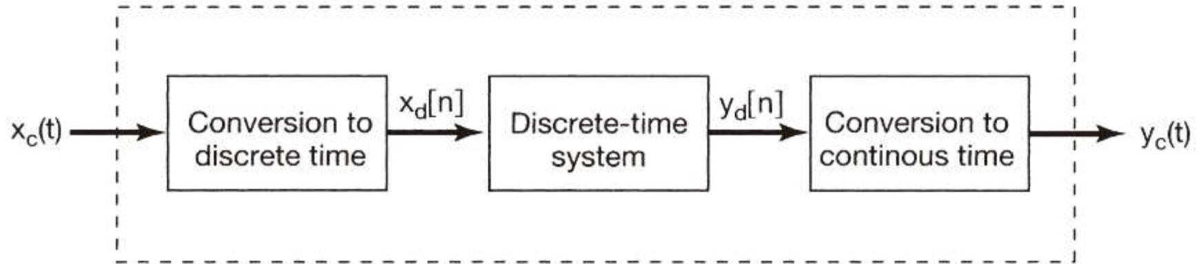
The transformation of  $x_c(t)$  to  $x_d[n]$  corresponding to the first system in Figure 7.19 will be referred to as *continuous-to-discrete-time conversion* and will be abbreviated C/D. The reverse operation corresponding to the third system in Figure 7.19 will be abbreviated D/C, representing *discrete-time to continuous-time conversion*.
