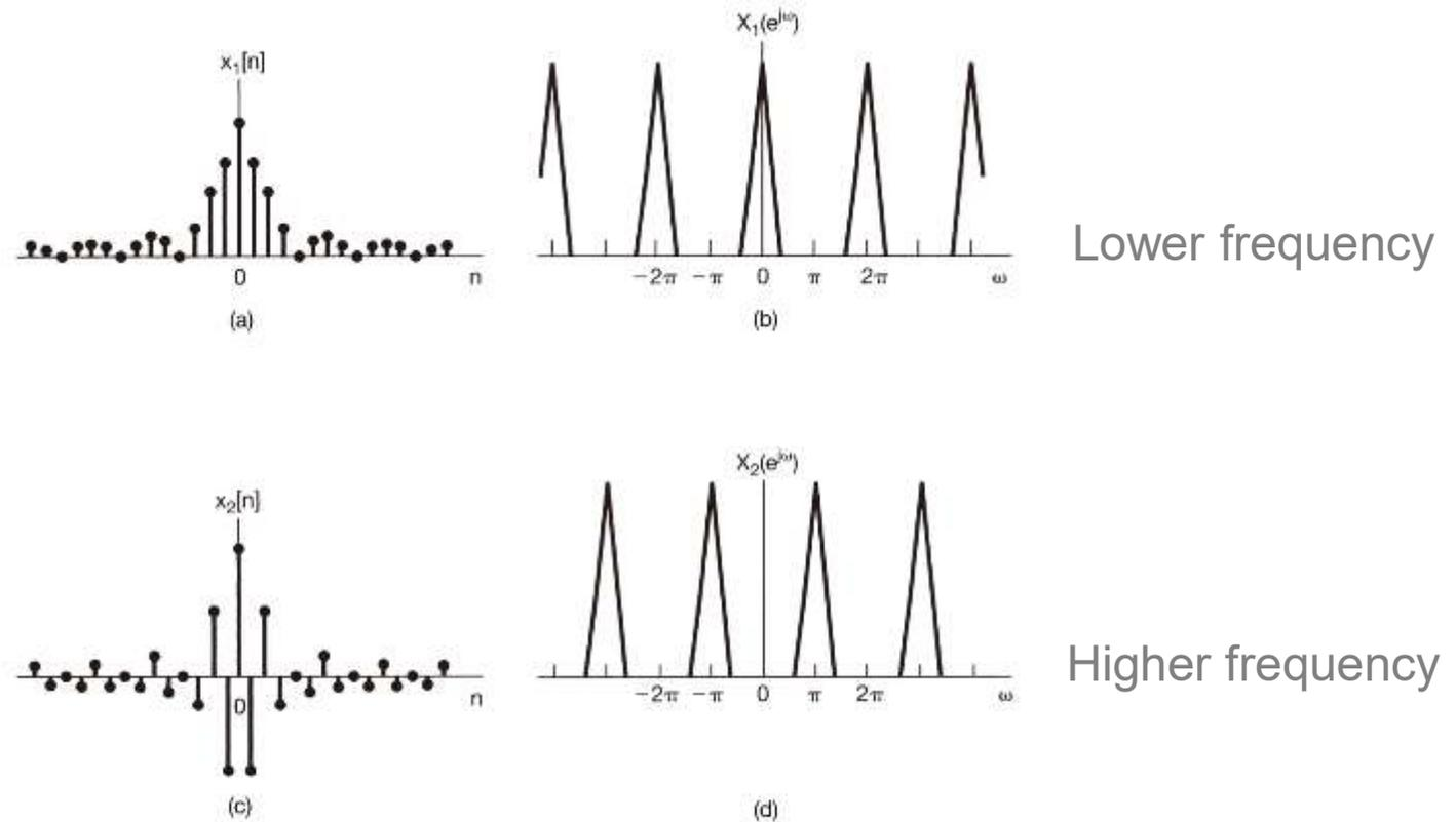
**Figure 5.3** (a) Discrete-time signal  $x_1[n]$ . (b) Fourier transform of  $x_1[n]$ . Note that  $X_1(e^{j\omega})$  is concentrated near  $\omega = 0, \pm 2\pi, \pm 4\pi, \dots$ . (c) Discrete-time signal  $x_2[n]$ . (d) Fourier transform of  $x_2[n]$ . Note that  $X_2(e^{j\omega})$  is concentrated near  $\omega = \pm\pi, \pm 3\pi, \dots$ .
