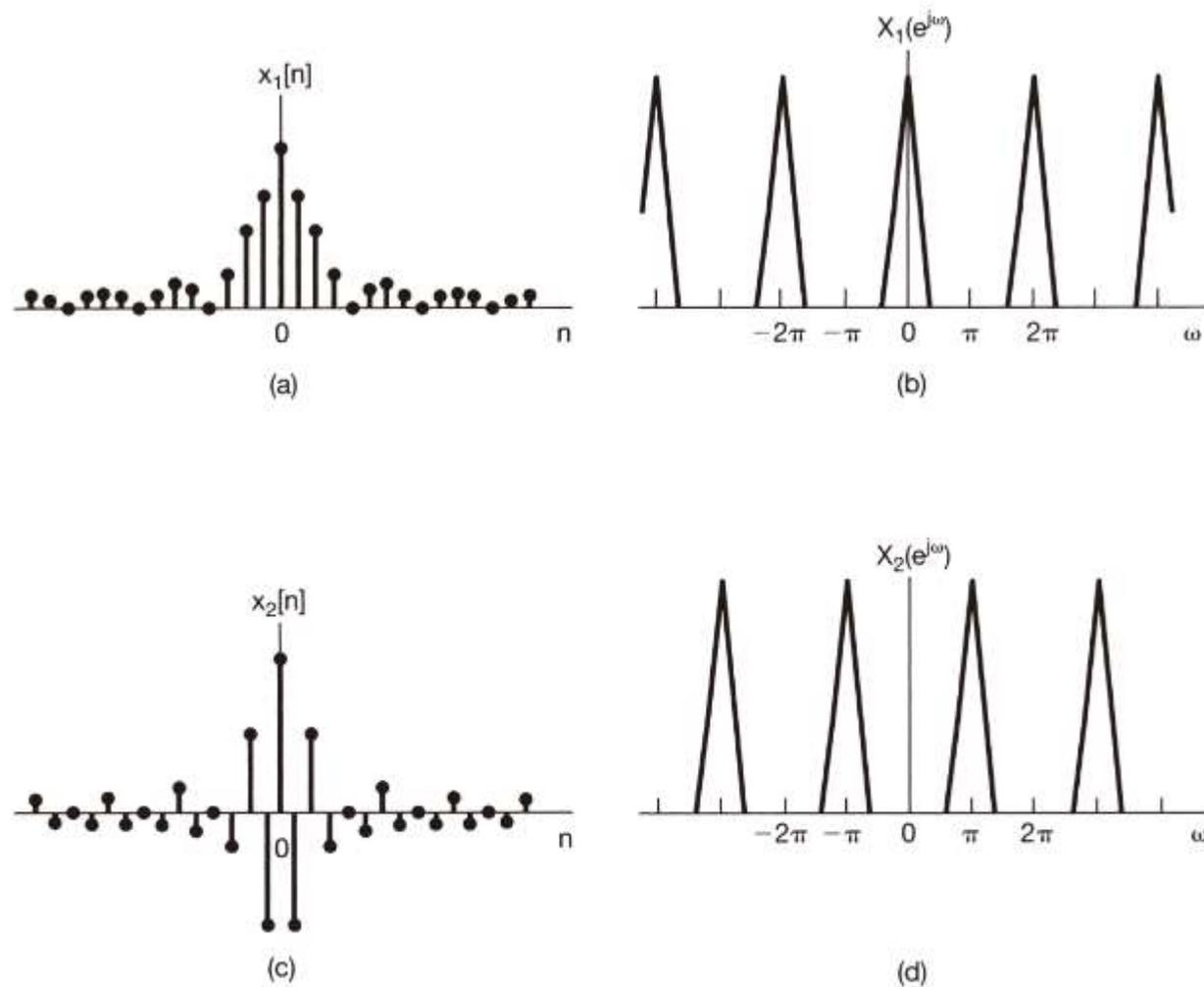
**Figure 5.3** (a) Discrete-time signal  $x_1[n]$ . (b) Fourier transform of  $x_1[n]$ . Note that  $X_1(e^{j\omega})$  is concentrated near  $\omega = 0, \pm 2\pi, \pm 4\pi, \dots$ . (c) Discrete-time signal  $x_2[n]$ . (d) Fourier transform of  $x_2[n]$ . Note that  $X_2(e^{j\omega})$  is concentrated near  $\omega = \pm\pi, \pm 3\pi, \dots$ .
