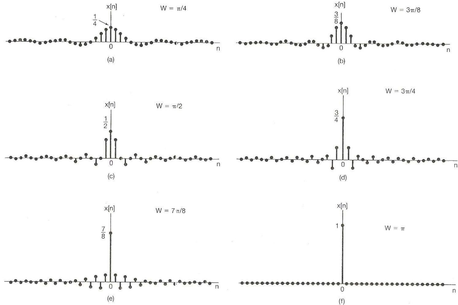
Figure 5.7 Approximation to the unit sample obtained as in eq. (5.16) using complex exponentials with frequencies  $|\omega| \leq W$ : (a)  $W = \pi/4$ ; (b)  $W = 3\pi/8$ ; (c)  $W = \pi/2$ ; (d)  $W = 3\pi/4$ ; (e)  $W = 7\pi/8$ ; (f)  $W = \pi$ . Note that for  $W = \pi$ ,  $\hat{x}[n] = \delta[n]$ .
