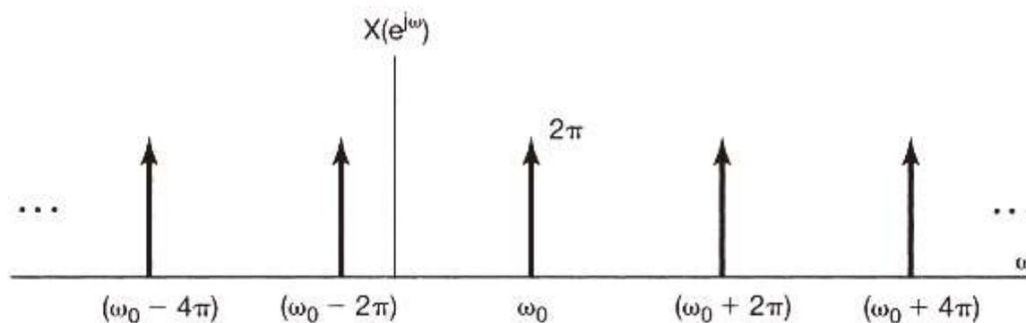
**Figure 5.8** Fourier transform of  $x[n] = e^{j\omega_0 n}$ .
