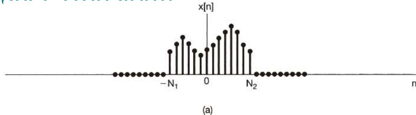
From this aperiodic signal, we can construct a periodic signal  $\tilde{x}[n]$  for which  $x[n]$  is one period, as indicated in Figure 5.1(b).
