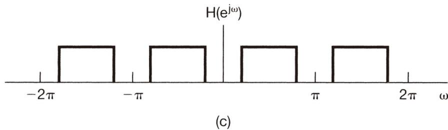
**Figure 3.28** Discrete-time ideal frequency-selective filters: (a) lowpass; (b) highpass; (c) bandpass.
