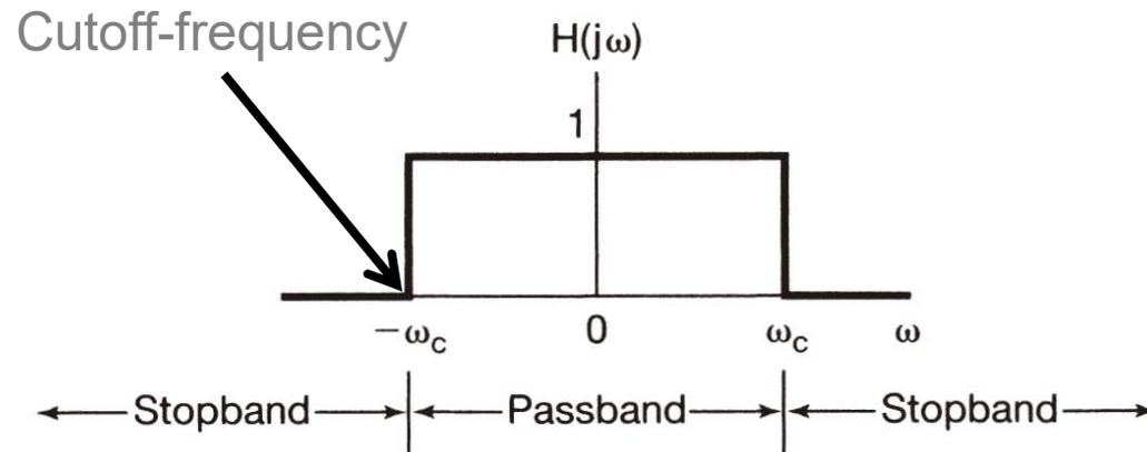
**Figure 3.26** Frequency response of an ideal lowpass filter.
