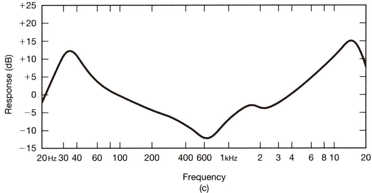
**Figure 3.22** Magnitudes of the frequency responses of the equalizer circuits for one particular series of audio speakers, shown on a scale of  $20 \log_{10} |H(j\omega)|$ , which is referred to as a decibel (or dB) scale. (a) Low-frequency filter controlled by a two-position switch; (b) upper and lower frequency limits on a continuously adjustable shaping filter; (c) fixed frequency response of the equalizer stage.
