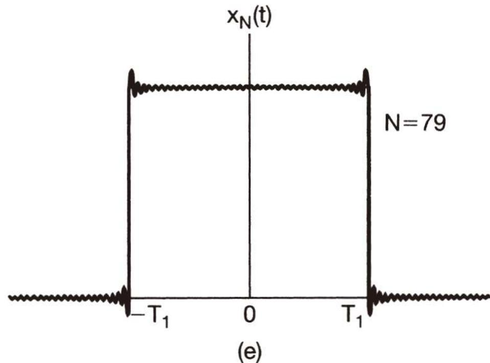
**Figure 3.9** Convergence of the Fourier series representation of a square wave: an illustration of the Gibbs phenomenon. Here, we have depicted the finite series approximation  $x_N(t) = \sum_{k=-N}^N a_k e^{jk\omega_0 t}$  for several values of  $N$ .
