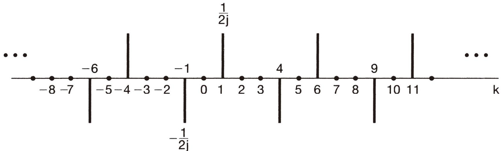
**Figure 3.13** Fourier coefficients for  $x[n] = \sin(2\pi/5)n$ .
