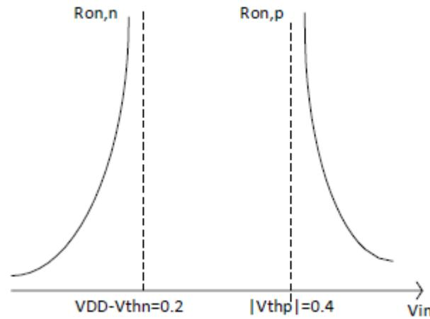
Comment : Both N/PMOS turn off when  $0.2 < V_{in} < 0.4$ , and  $R_{on} \rightarrow \infty$
