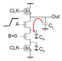
Solution: add secondary pre-charge transistors : typically need to pre-charge every other node, Big load capacitance CY helps as well.
