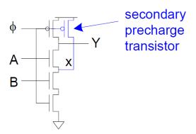
(C)Susceptible to crosstalk due to 1) high impedance of the output node and 2) backgate capacitive coupling
