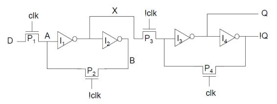
(a) direct path from D to Q during the short time when both clk and !clk are high (1-1 overlap)
