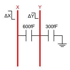
$$\Delta Y = \Delta X \times \left(\frac{C_{adj}}{C_{adj} + C_{gnd}}\right) = 1 \times \frac{2}{3} = \frac{2}{3}$$
