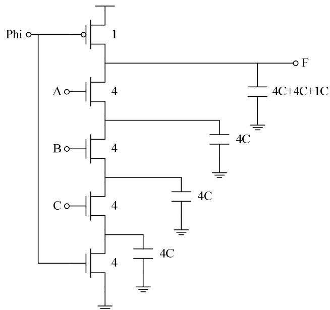
Let  $V_x$  be the voltage at node F which is suffered from charge sharing.
