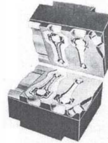
Closed forging dies used to produce an automobile connecting rod.
