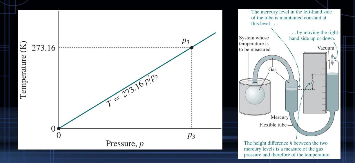
Triple point of water: Liquid water, solid ice, and water vapor (gaseous water) can coexist, in thermal equilibrium, at only one set of values of pressure and temperature. The triple point of water has been assigned a value of 273.16 K
