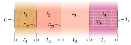
Assuming the conduction rate of each section is  $P_1, P_2, P_3, P_4$ . Since the heat flow is steady, then we have  $P_1 = P_2 = P_3 = P_4$ .
