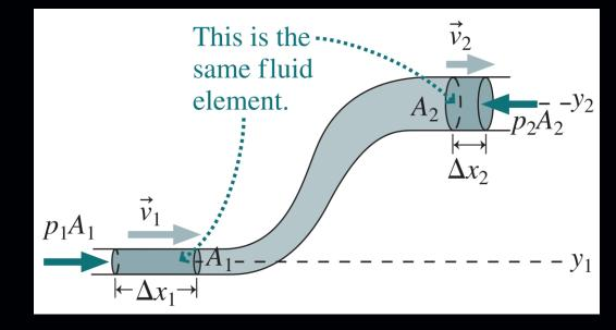
• The change of gravitation energy:  $W_g = mg(y_2 - y_1)$ . • The change of kinetic energy:  $\Delta K = \frac{1}{2}m(v_2^2 - v_1^2)$ With work energy theorem:  $W1 + W2 + W_g = \Delta K$ We have  $p_1A_1\Delta x_1 - p_2A_2\Delta x_2 + mg(y_2 - y_1) = \frac{1}{2}m(v_2^2 - v_1^2)$
