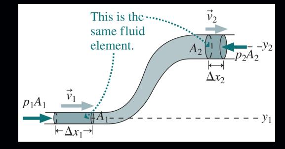
Consider the conservation of energy in fluid motion: the same fluid element flow from one side to the other side:
