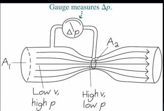
The venturi flow : Measuring the pressure difference between the constricted and the unconstricted pipe gives a measure of the flow speed.
