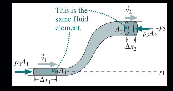
Neglecting fluid friction (viscosity) and in the absence of mechanical pumps and turbines that add or remove energy from the incompressible fluid, Bernoulli's equation reads
