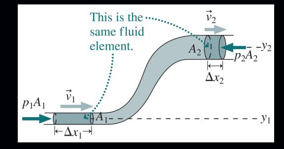
Since volume V=A∆x and m/V=p, plug in to the previous equation we get:
