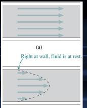
Without viscosity, flow in a pipe would be uniform. Viscous drag at the pipe walls introduces a parabolic flow profile.
