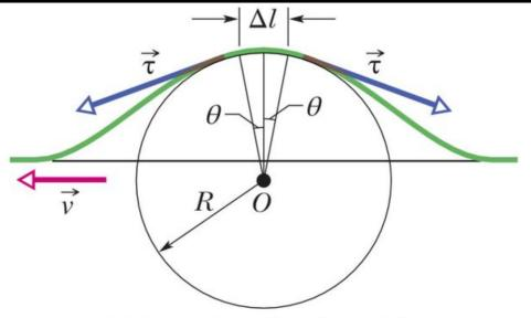
A radial restoring force with magnitude  $F = 2\tau sin\theta \approx \tau \frac{\Delta l}{R}$ The mass of the element is  $\Delta m = \mu \Delta l$ , where  $\mu$  is the unit mass of the string.
