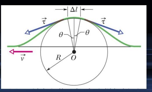
Consider a small string element of length  $\Delta I$  within the pulse, an element that forms an arc of a circle of radius R and subtending an angle 20 at the center of that circle. A force  $\vec{\tau}$ with a magnitude equal to the tension in the string pulls tangentially on this element at each end.
