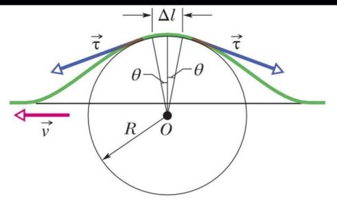
Considering it as a uniform circular motion, the force provide a centripetal acceleration: $a = \frac{v^2}{R}$  to the mass  $\Delta m = \mu \Delta l$ . Thus, we have  $\tau \frac{\Delta l}{R} = \mu \Delta l a = \mu \Delta l \frac{v^2}{R}$ There fore we can get  $v = \sqrt{\frac{\tau}{\mu}}$ , which is the wave speed of the stretched string.
