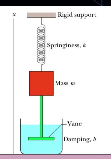
Let us assume the liquid exerts a damping force  $\overrightarrow{F_d}$  that is proportional to the velocity  $\vec{v}$  of the vane and block (an assumption that is accurate if the vane moves slowly). Then, for force and velocity components along the x axis in we have  $F_d = -bv$ where b is a damping constant.
