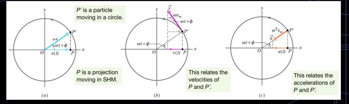
Simple harmonic motion is the projection of uniform circular motion on a diameter of the circle in which the circular motion occurs.
