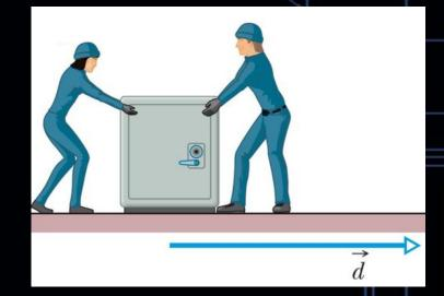
(a) What is the net work done on the safe by forces  $\overrightarrow{F_1}$  and  $\overrightarrow{F_2}$  during the displacement ? The work done by  $\overrightarrow{F_1}$  is  $W_1 = F_1 \cdot d \cdot \cos 30^\circ = 88.3I$ and the work done by  $\overrightarrow{F_2}$  is  $W_2 = F_2 \cdot d \cdot \cos 40^\circ = 65.1J$ Thus, the net work W  $W = W_1 + W_2 = 153.4J$
