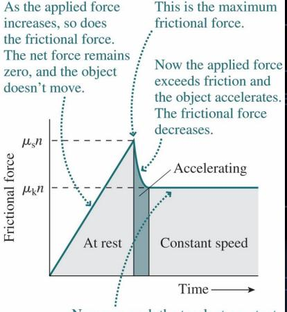
Now you push the trunk at constant speed, so your applied force is equal in magnitude to the lower force of kinetic friction.
