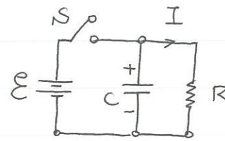
loop rule:  $V_C = IR = \frac{Q}{C}$ , where  $Q$  is the charge on  $C$ .
