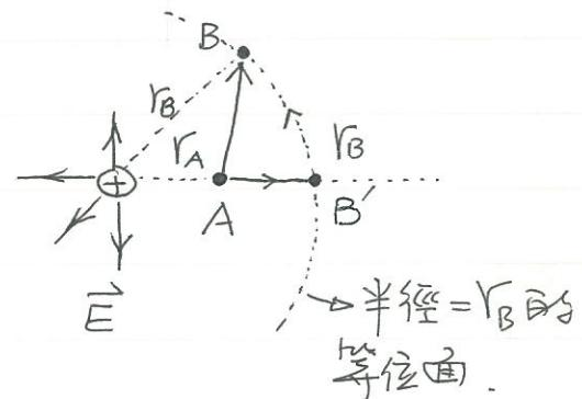
$$\begin{aligned} \therefore \Delta V_{AB} &= \int_A^{B'} \vec{E} \cdot d\vec{r} = - \int_{r_A}^{r_B} \frac{kq}{r^2} \cdot \hat{r} \cdot dr = -kq \int_{r_A}^{r_B} \frac{dr}{r^2} \\ &= kq \left( \frac{1}{r_B} - \frac{1}{r_A} \right) = V_B - V_A \end{aligned}$$
