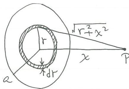
$$\begin{aligned} d\sigma &= \text{半徑 } r \text{ 寬度 } dr \text{ 的 ring 所帶 charge} \\ &= \sigma \cdot dA \quad (dA = \text{ring 的面積}) \\ &= \sigma \cdot 2\pi r \cdot dr, \text{ where } \sigma = \frac{Q}{\pi a^2} = \text{surface charge density} \end{aligned}$$
