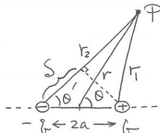
$$V(p) = \sum \frac{k\delta_i}{r_i} = \frac{k\delta}{r_1} - \frac{k\delta}{r_2}$$
