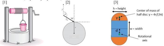
[1] A bucket of mass m drops into a well, its rope unrolling from a cylinder of mass M and radius R. What's its acceleration? (Express your answer as a function of m, M, g)
