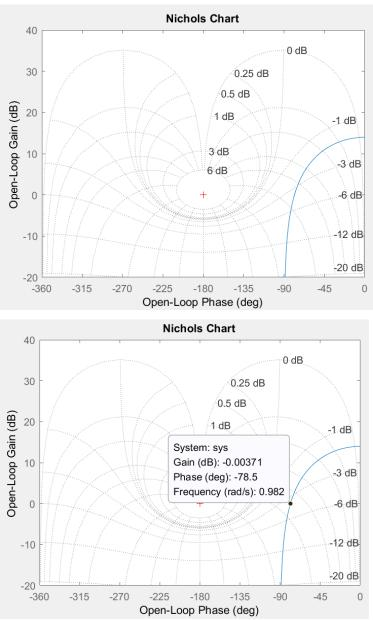
Gain margin: The plot reaches  $-180^{\circ}$  at infinite frequency (GM =  $\infty$ ) Phase margin: PM =  $101.5^{\circ}$
