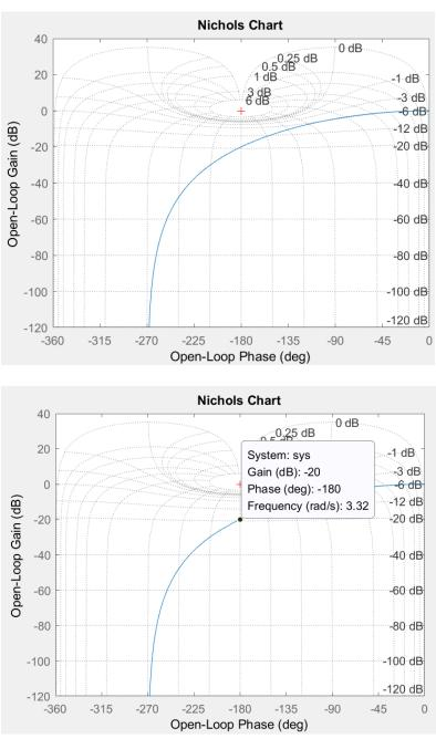
Gain margin: -20dB Phase margin: The plot reaches 0dB at infinite frequency (PM =  $\infty$ )
