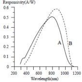
2. Figure below shows the responsivity of an InAs pn junction photodiode to use in the infrared. It is normally cooled under normal operation. (a) What is the wavelength and the quantum efficiency at the peak responsivity at -40 degree C? (b) The diode area that is involved in the detection as a diameter of 0.25 mm. What is the intensity of light that corresponds to a photocurrent of 50 nA?
