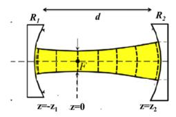
Consider the optical cavity shown in the diagram below in which the variation of the spot size w(z) is also shown. Note that the beam waist occurs at a distance d to the left of M1 and that the mirrors have curvature of opposite signs.
