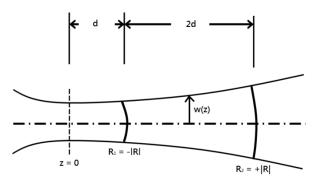
(a) Assume that the cavity is stable. Solve for the ratio d/R and evaluate the parameter  $z_0^2$ .
